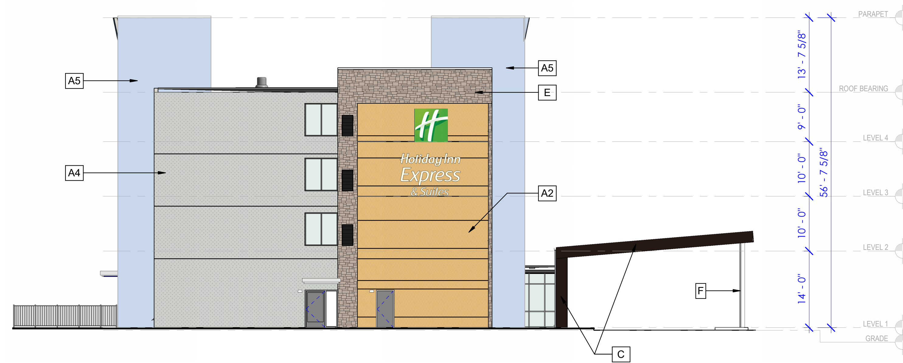
EXTERIOR ELEVATION EAST SCALE: 3/32" = 1'-0"
